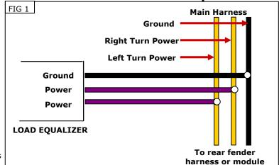
access is beneath the seat or behind a side cover. Cut off the connector of the included load equalizer and using the included Scotch Locks, connect one violet wire from the load equalizer to the bikes' right turn power wire and the other violet wire from the load equalizer to the bike's left turn power wire. Connect the black wire from the load equalizer to the ground wire. FIG 1
